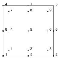
Figure 3-34 Integration Points of Eight-node, 2-D Element
