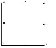
Figure 3-33 Nodes of Eight-node, 2-D Element
